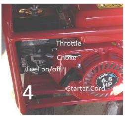
Turn the electrical switch on the side of the engine to on. Turn on the fuel from the lever at the end of the engine and apply the choke with the lever below the fuel lever. Start the engine by pulling the starter cord.
