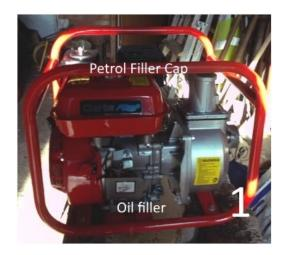
Check the fuel level. The fuel filler cap is located on the fuel tank fitted above the engine. The pump engine runs on unleaded petrol. Petrol is stored in the fuel store located adjacent to the lifting gantry at the down river end of the boat shed.
